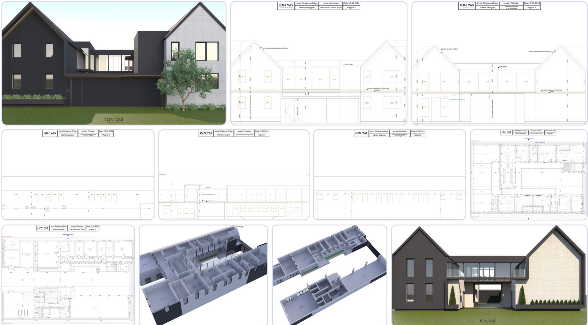
Elevations, sections and floor plans of a single-storey smart house with an annex; 3D massing model; the black-and-white render of the twin-gable concept.
